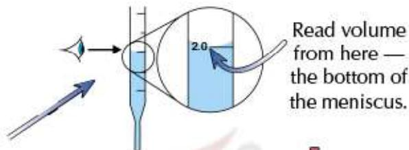
**Pipettes** are long, narrow tubes that are used to suck up an **accurate** volume of liquid and **transfer** it to another container. A **pipette filler** attached to the end of the pipette is used so that you can **safely control** the amount of liquid you're drawing up. Pipettes are often **calibrated** to allow for the fact that the last drop of liquid stays in the pipette when the liquid is ejected. This reduces **transfer errors**.
